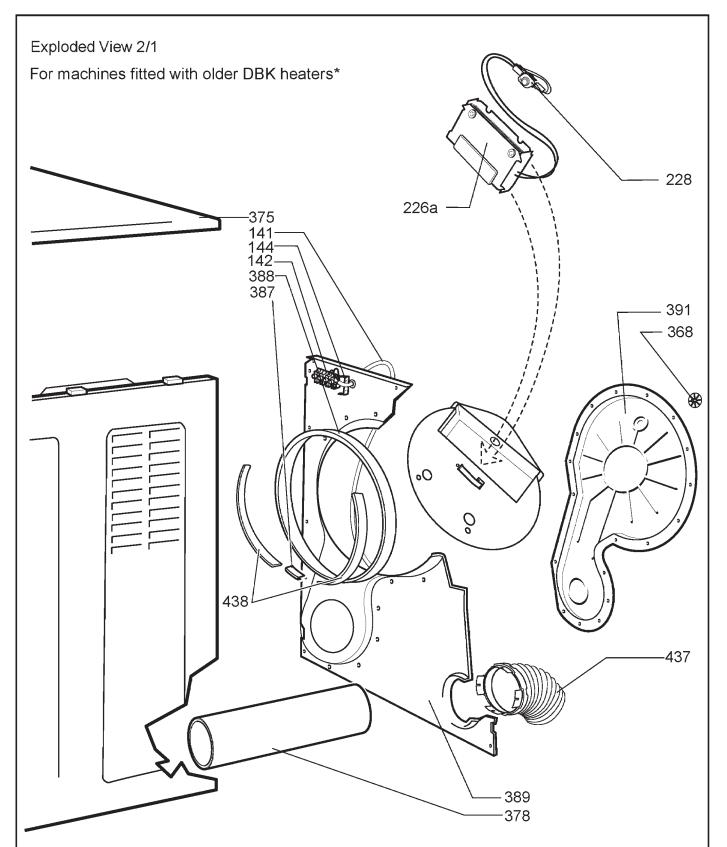
\*DBK heaters (item 226a) have now been replaced by new sheathed heaters (see exploded view 2/2). Please refer to the parts list for details of when the new heaters were introduced.
